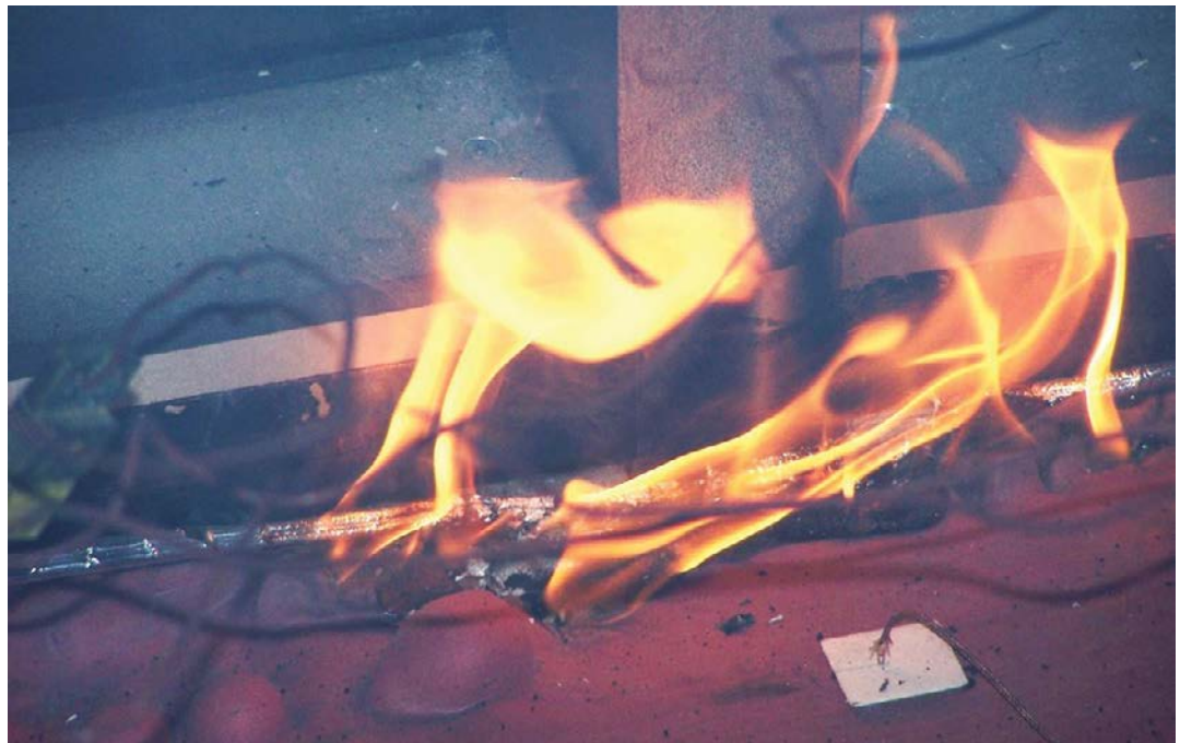
A failed ASTM E2307 fire test—flame spread through safing gap (having insulation and sealant) due to curtain wall reaction to fire exposure.
