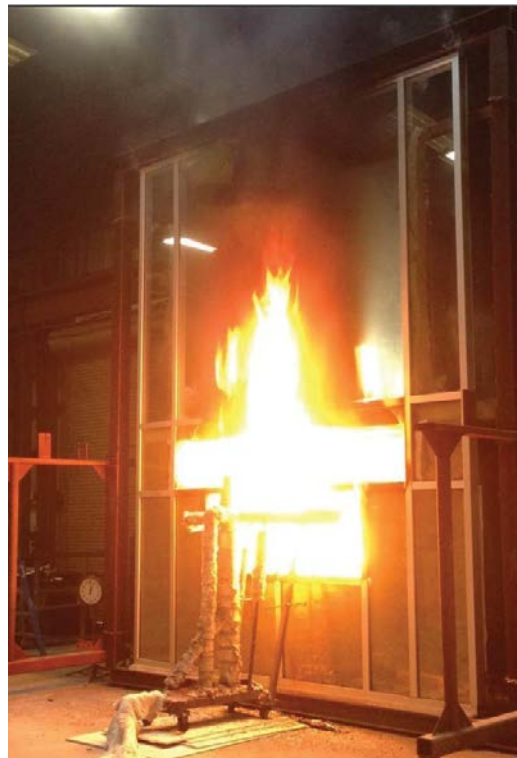
ASTM E2307 fire test after ignition of exterior burner (at five minutes).
