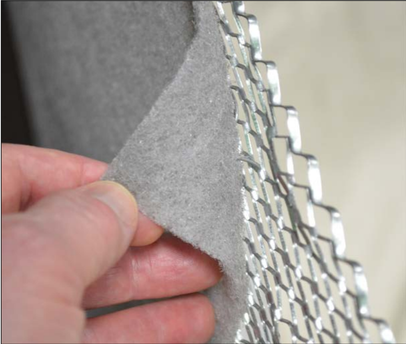
A factory-assembled metal lath and drainage plane system for adhered masonry.
